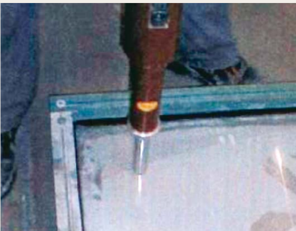
Point 1 – Edge Impact with Concrete Testing Hammer
