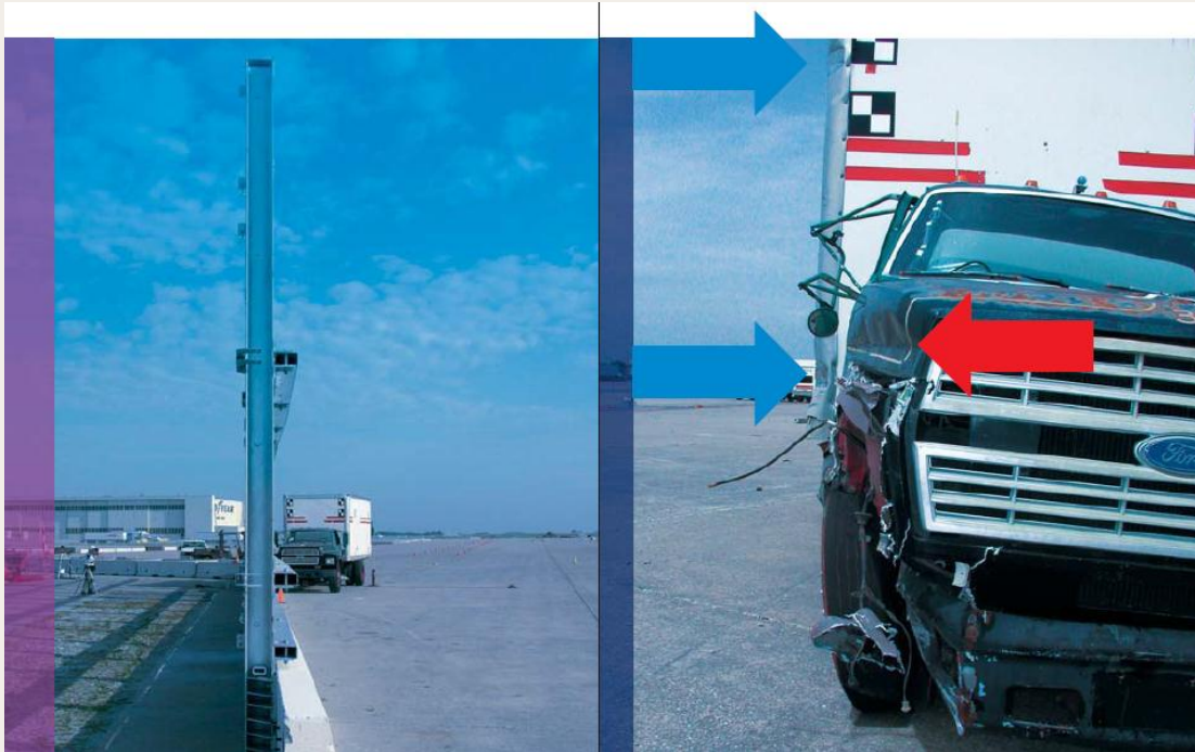
18,000 pound truck impacts the TL4 System at 50 MPH and at an angle of 15°
