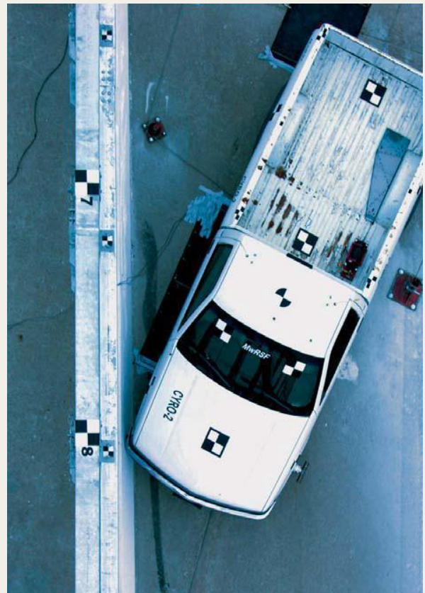
A 4,400 lb pickup truck impacts the TL4 System at 60 mph at a 25° angle
