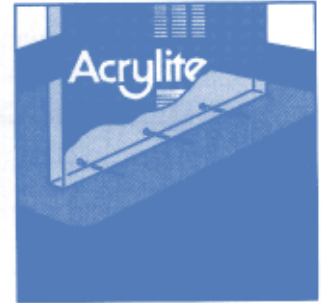
Soak cementing. Material must be supported on pins or wire brads. See page 20.
