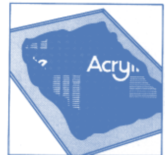
Roll the masking paper back about 1/2" to allow work on the edges of the sheet.
