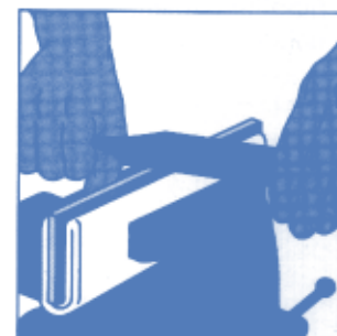
Slide the file at an angle to prevent cutting grooves into your work.
