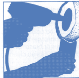
Always use a buffing compound for polishing. Use it sparingly.
