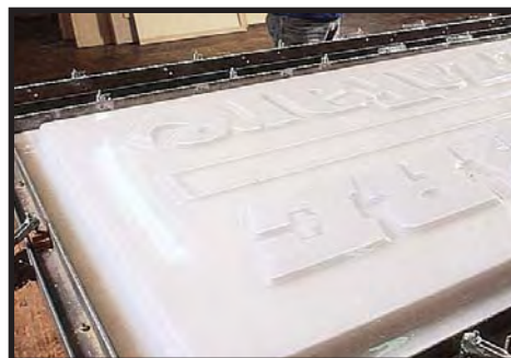
Immediately after thermoforming, the sheet will appear a milky white color. Cooling cycles can be reduced by using cooling fans or applying compressed air.
