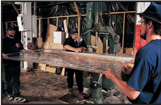
Bandsaw cutting is easily accomplished with ACRYLITE SG sheet.
