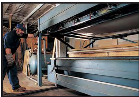
Ideal thermoforming temperature is between 310 - 320°F. Many thermoformers judge readiness by the sag and the feel of the sheet.
