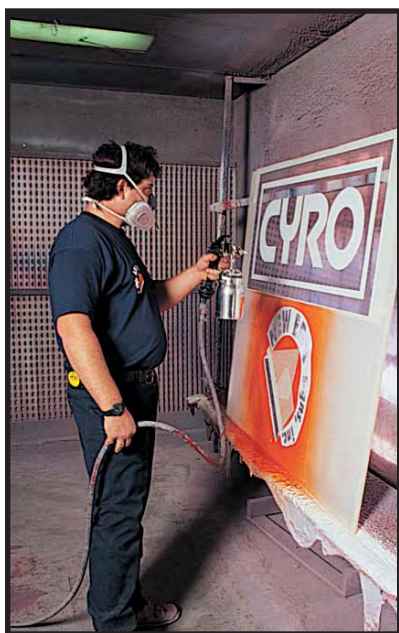
Painting techniques typically used with acrylic and polycarbonate sheet can be used with ACRYLITE SG sheet.
