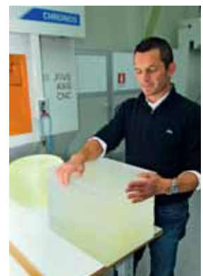
Scacchi layers one sheet of ACRYLITE® on another. The individual sheets are bonded into a block, from which the vase is made.
