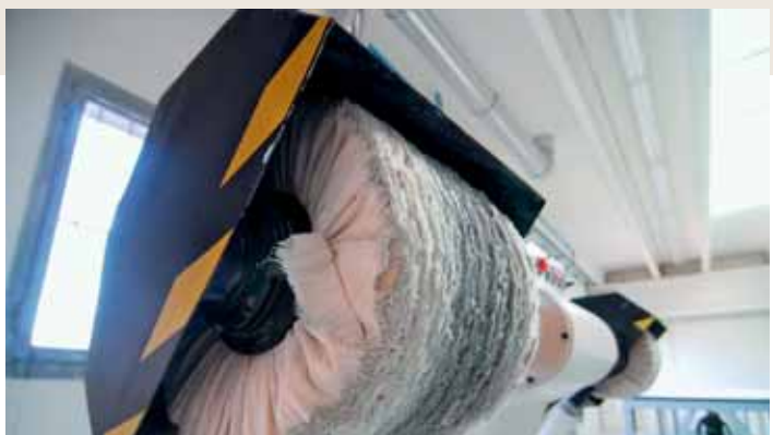
Smooth and glossy: what looks like part of a washing machine is the polishing unit that gives the vases the finishing touch. After that they appear like noble exhibits with an amber sheen.
