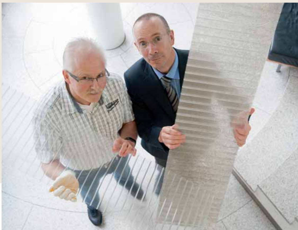
Martin Berkenkopf (on right), Product Manager at Acrylic Polymers, shows how a sheet covered in algae may look after several years of service. Wolfgang Scharnke, Technical Project Manager for "AAA" holds up a clean sheet for comparison.
